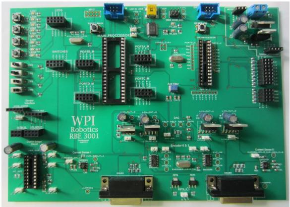
The RBE Development board is designed to use an AVR644P to control a robotics system. The Board has multiple functions and features.
